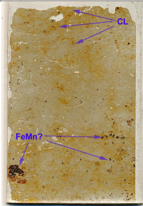
Fig. 21: Scan of M1; massive, bedded and laminated loamy silts (Figs 22-24), with micritic impregnations, patchy iron staining, inwashed clay (CL; Figs 24-29) and secondary iron-manganese nodular impregnations probably linked to later rooting (FeMn?). Frame height is 90mm.
