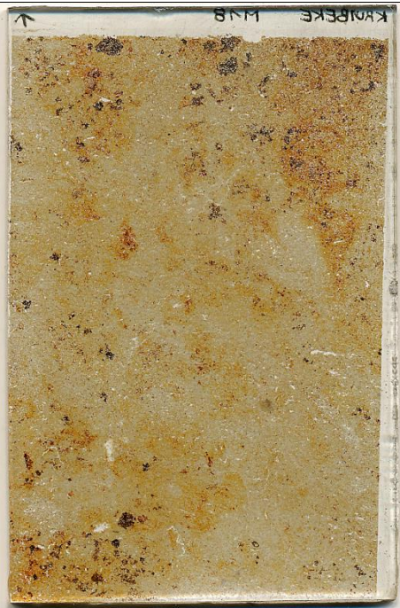
Fig. 6: Scan of M18; massive decalcified silty fine sands and fine sandy silt loams, showing iron mottling, often associated with clay void coatings (Figs 7-11); some root traces are picked out by probable iron-manganese nodules. Frame height is ~90mm.
