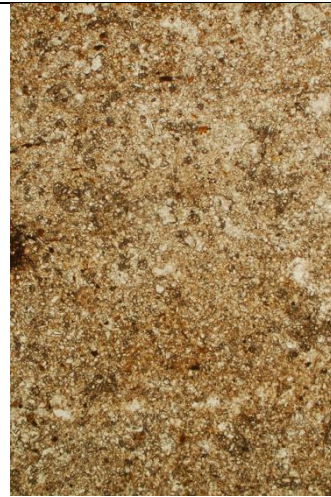
Fig. 22: Photomicrograph of M1; relict sedimentary layers and laminae composed of loamy silts and very fine sands. PPL, frame height is ~4.62mm.
