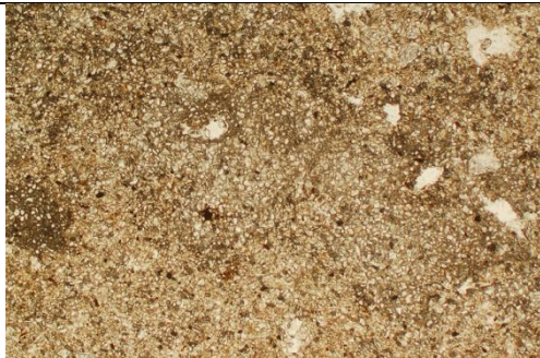
Fig. 4: Photomicrograph of M21; probably fine rooted silts with associated (dark grey) micritic calcium carbonate impregnations. PPL, frame width is ~4.62mm.
