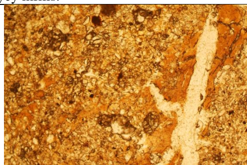
Fig. 30: Photomicrograph of M1; another example of clay inwash. PPL, frame width is ~2.38mm.
