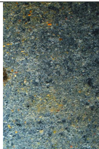
Fig. 24: As Fig 22, under OIL; note very weak iron staining.
