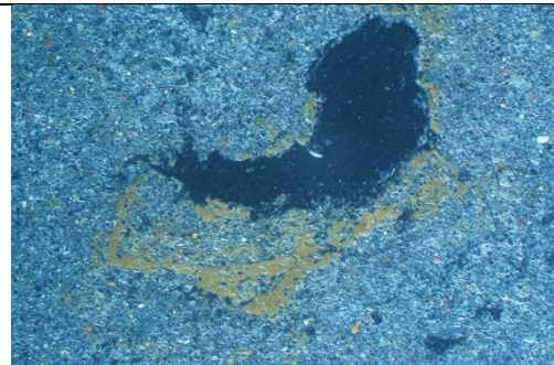
Fig. 3: As Fig 2, under oblique incident light (OIL), illustrating clay inwash.
